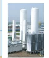
tank blanketing Location: ECOVAR® solution: CRYOSS®-N Capacity: 2 x 1,200 Nm³/h nitrogen Installation date:
